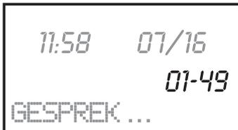
during a call, the display will indicate the elapsed call duration; immediately after disconnecting the call, this timer will disappear
