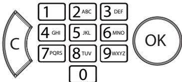
use the **C** button to delete the incorrect number, enter the correct number and press the **OK** button
