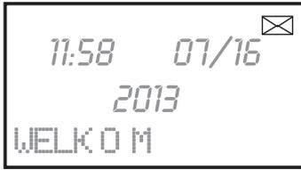
If your telephone service provider supports the Voicemail service, based on the FSK system, then it's possible that you receive a notification when somebody has left you a new message. In the upper right corner of the display the ☒ symbol will be shown. The DTMF system doesn't support this indication.
